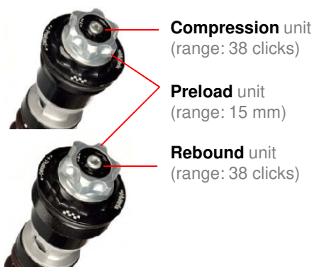
F20K fork kit quad-valve asymmetric system
